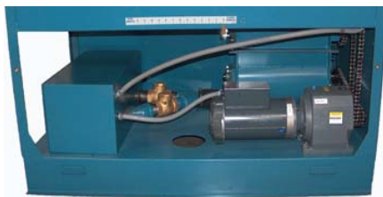
2 HP Direct Drive Motor/Reducer for Increased Torque/ Reduced Amperage
